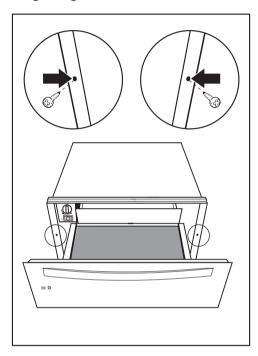
Open the drawer and fix the appliance with the two supplied screws at the side panels of the cabinet. The installation kit contains 3 metal strips with adhesive on the back side.
